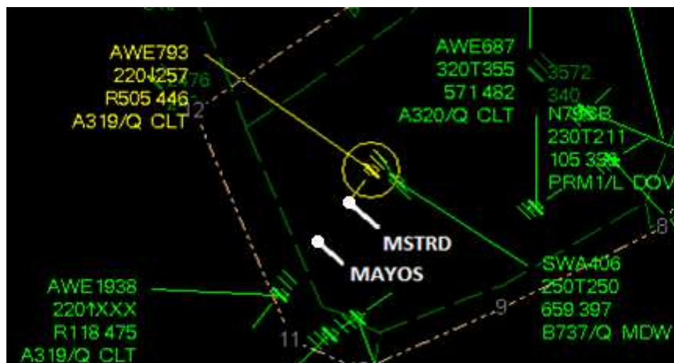
Figure 7: Actual Loss of Separation involving Airbus FMS, MSTRD restriction was FL 260 (Image courtesy Washington ARTCC)
